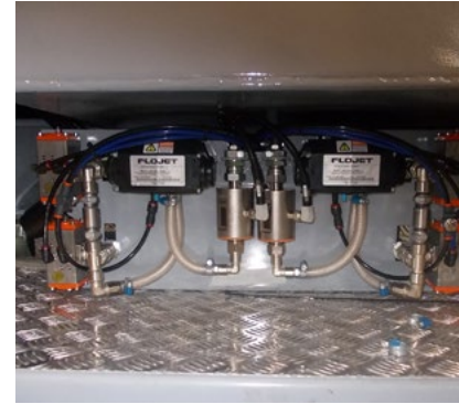
Flow sensor for liquid additives dosing
