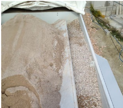
Mobile adjustable bulkhead for the sand compartment
