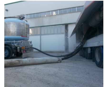
Pneumatic refilling system for cement compartment
