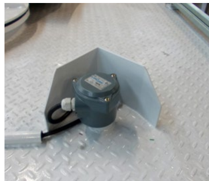
Level sensor on the binder compartment with alarm siren
