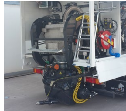
Pre-mixer on load cells
